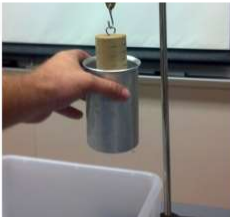
Figure 2. Taking data for Part 3. The object is lowered into a cup of water until it reached the desired line. The force recorded by the sensor is less than the weight of the block in the air because the buoyancy force supports the object.
