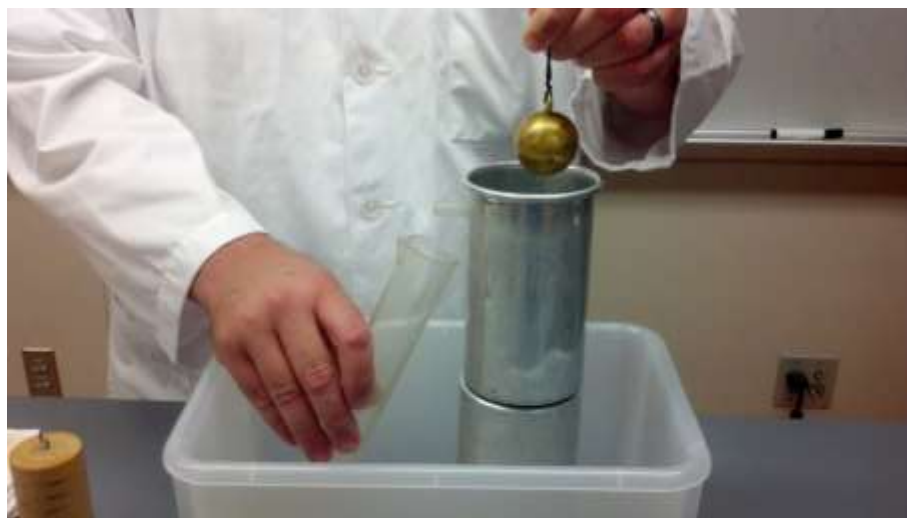
Figure 1. Ready to perform Part 1. The upper container (with the spout) was set in place, and then it was "topped off" with water. (The extra water fell into the plastic bin.) The graduated cylinder is ready to catch the overflow that will come out when the brass ball is lowered into the water. (Do not copy our picture into your lab report!)
