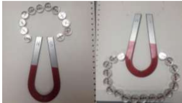
Figure 1. Horseshoe magnet with compasses measuring the magnetic field direction.
